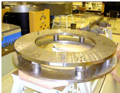
图9 FMD (力测量设备) Fig.9 Force measurement device
