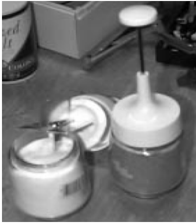
图6 粉末阻尼器样机 Fig.6 Prototype of a powder damper
