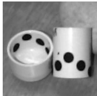
图 5 Velcro 阻尼器样机 Fig.5 Prototype of a velcro damper
